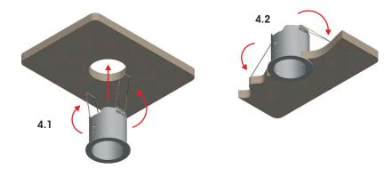
5 Insert the fixture though the installed base and turn it clockwise to lock it in desired position.
