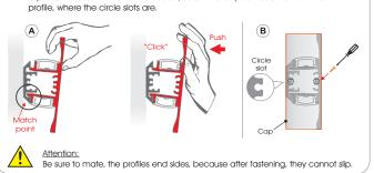
7 A. To unfasten the luminaire-profile from its place, unscrew the caps on each side and remove them.
