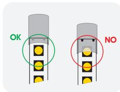
4 Remove gradually the masking tape and stick the led strip on the desired surface.
