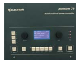
User interface using Keyboard, 128x64 dot matrix display, and two encoders for easy programming
